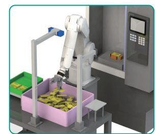
Picking from a large pallet (Fixed camera)
